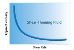
The viscosity of a grease changes when sheared. Apparent Viscosity, reported in centipoise, gives a design engineer an indication of the "shear quality" of a grease at specific temperatures. (Water is about 1 cP. Wood putty is about 1 million cP.)
